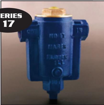
The No.17 Float and Thermostatic Trap is recommended for steam mains, branches, and risers where a relatively small volume of condensate is encountered.
